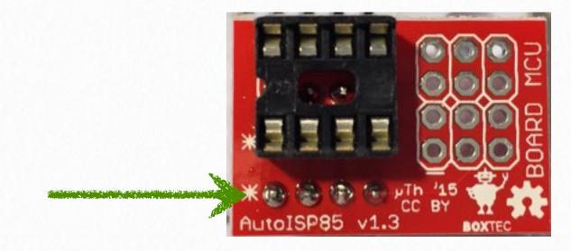
4. Insert the two 2x3 pin male headers from the **top** of the board and solder on the bottom.
