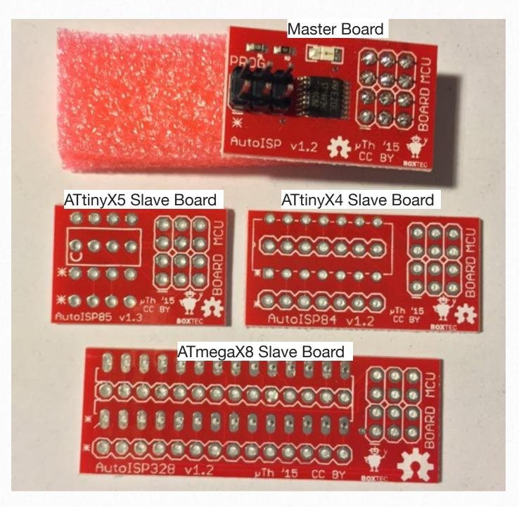
AutoISP is a development system to facilitate programming microcontrollers through the SPI serial protocol. It consists of a universal master board containing the logic, plugged into one of a family of slave boards containing the wiring for a particular microcontroller
