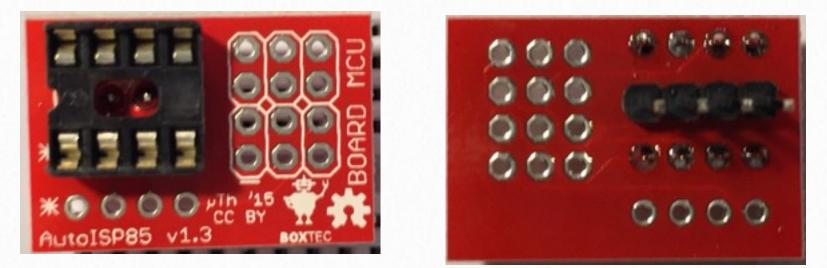
3. Insert the other single row male header strips from the **bottom** of the board into bottom row of holes, and solder it on top.
