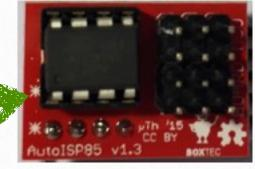
3. Plug AutoISP master board into the slave board, such that the two boards are in parallel and the labels "AutoISP", "MCU" and "BOARD" appear in the same orientation on both boards.
