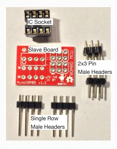
1. Insert one of the single row male header strips from the **bottom** of the board into the row of holes in the **middle** of the IC socket outline of the slave board, and solder it on top. The pins should extend only minimally (1-2mm) from the surface of the board. Make sure that all contacts are properly soldered, as the solder points will no longer be accessible after the next step (which is also why it's **crucial to perform this step first**).
