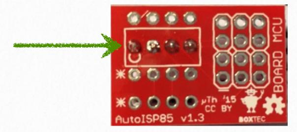
2. Insert the IC socket from the **top** of the board and solder it on the bottom (aren't you glad now you already soldered the middle row of pins?).
