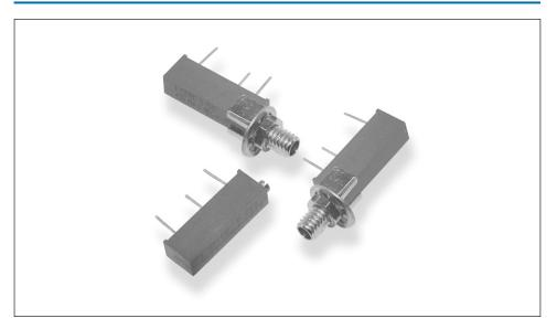
When you need a durable trimming potentiometer, these 19mm rectilinear styles offer quality performance at a competitive price. They feature a cermet element for stability and resolution and are available in two formats. Type 433 PW will withstand all recognised board-washing solvents and can be offered with panel mount for external adjustment.
