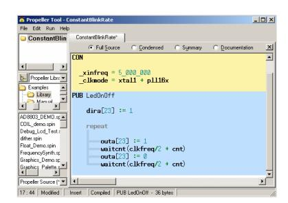
Click on **File** and save the program as "**ConstantBlinkRate**." Switch on your Protoboard and press **F11** to send the program to your Propeller. The LED should be flashing on and off.
