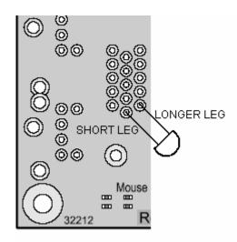
Normally we would insert a part into the holes and solder the connections on the bottom side. Since the holes we are using are intended for something else, just carefully insert the LED as shown.
