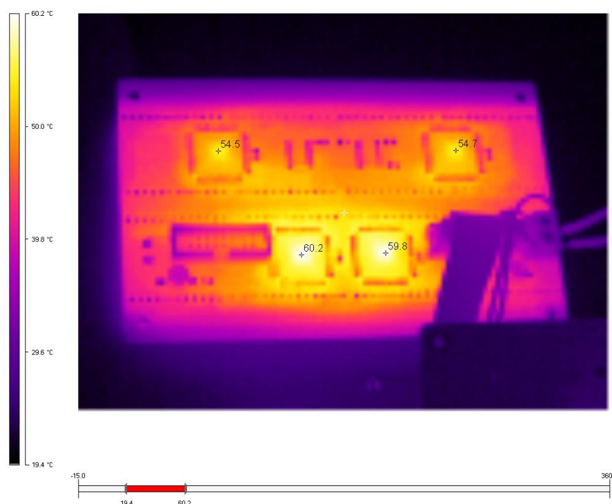
FIGURE 5-2 HEAT DISTRIBUTION OF THE BACK PANEL
