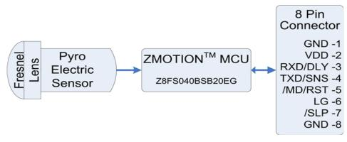
Figure 1. ZMOTION<sup>™</sup> Block Diagram
