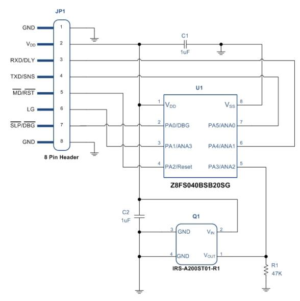
Figure 10. Schematic of ZMOTION<sup>™</sup> Detection Module
