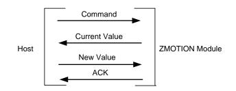
Figure 6. Write Command Structure
