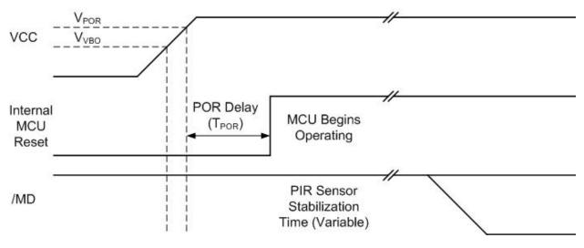
Figure 3. Power-On Reset Operation
