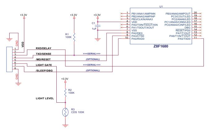
Figure 12. Application Example - Serial Interface Mode
