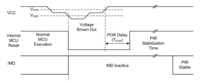
Figure 4. Voltage Brownout Reset Operation
