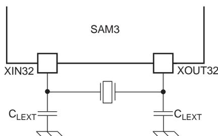
$$C_{LEXT} = 2x(C_{CRYSTAL} - C_{para} - C_{PCB}).$$
