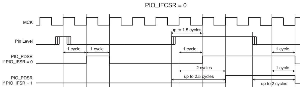
**Figure 32-6.** Input Debouncing Filter Timing
