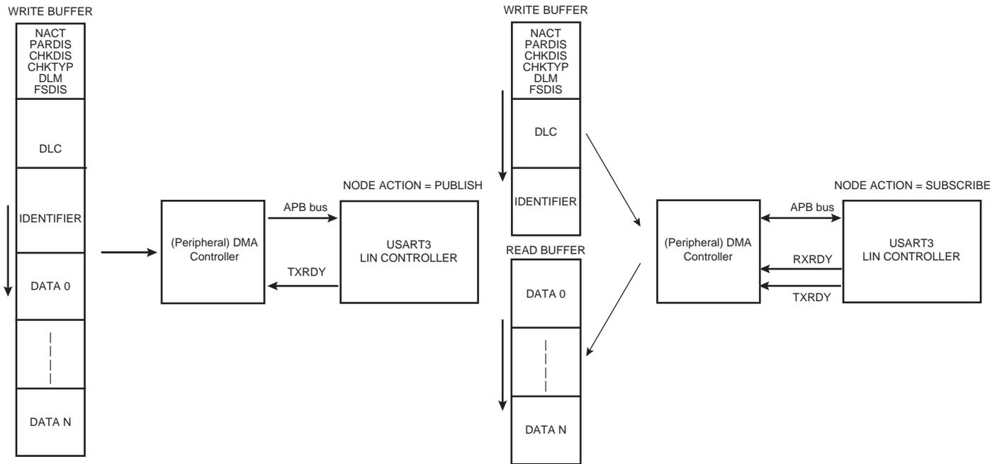
**Figure 36-53. Master Node with PDC (PDCM = 0)**
