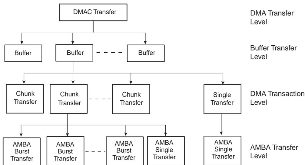
**Figure 24-3.** DMAC Transfer Hierarchy for Memory
