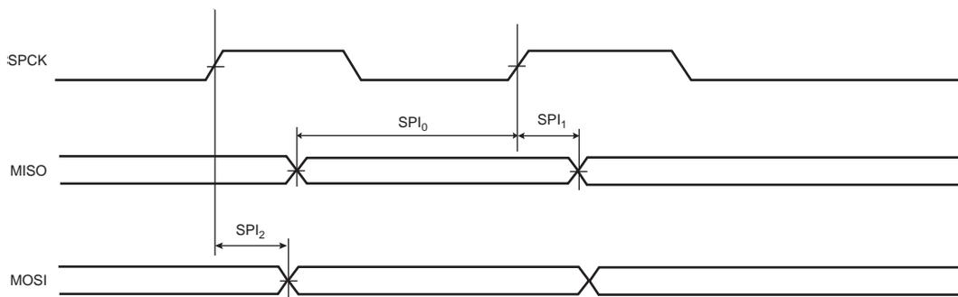
**Figure 46-16.** SPI Master Mode with (CPOL = 0 and NCPHA=1) or (CPOL=1 and NCPHA= 0)
