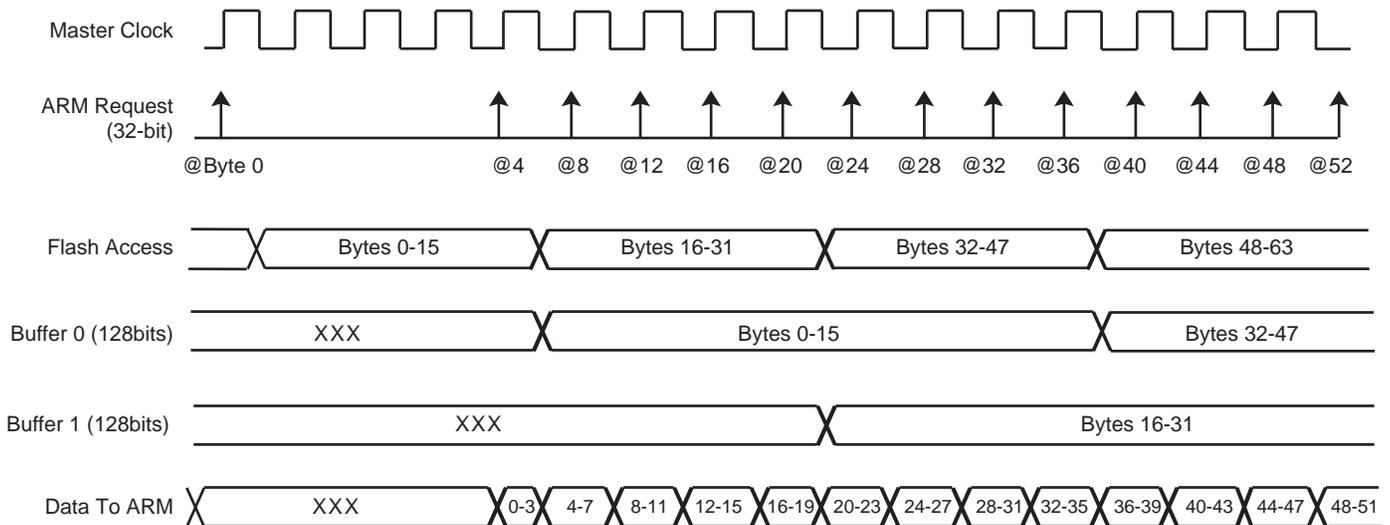
Note: When FWS is included between 1 and 3, in case of sequential reads, the first access takes (FWS+1) cycles, the other ones only 1 cycle.
