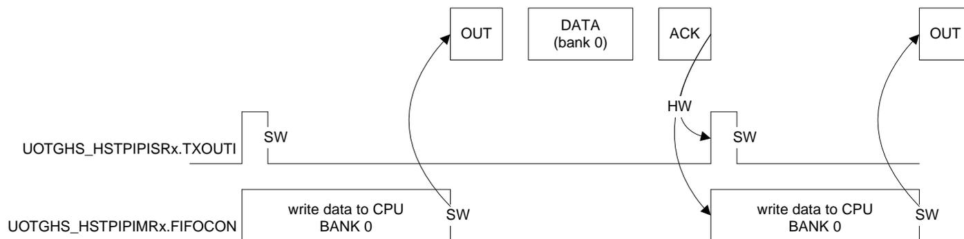
**Figure 40-27.** Example of an OUT Pipe with two Data Banks and no Bank Switching Delay
