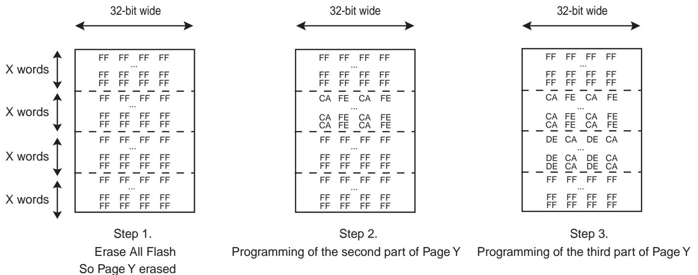
The Partial Programming mode works only with 128-bit (or higher) boundaries. It cannot be used with boundaries lower than 128 bits (8, 16 or 32-bit for example).
