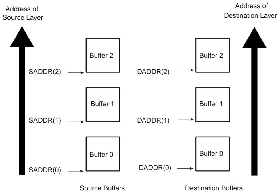
If the user needs to execute a DMAC transfer where the source and destination address are contiguous but the amount of data to be transferred is greater than the maximum buffer size `DMAC_CTRLAx.BTSIZE`, then this can be achieved using the type of multi-buffer transfer as shown in [Figure 24-6 on page 362](#).
