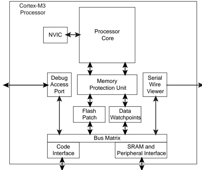
The Cortex-M3 processor is built on a high-performance processor core, with a 3-stage pipeline Harvard architecture, making it ideal for demanding embedded applications. The processor delivers exceptional power efficiency through an efficient instruction set and extensively optimized design, providing high-end processing hardware including single-cycle 32x32 multiplication and dedicated hardware division.
