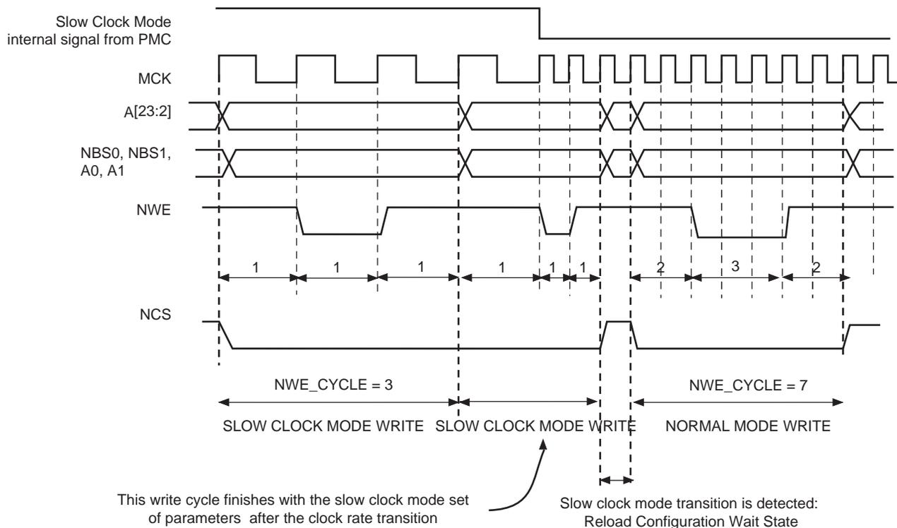
**Figure 27-30.** Recommended Procedure to Switch from Slow Clock Mode to Normal Mode or from Normal Mode to Slow Clock Mode
