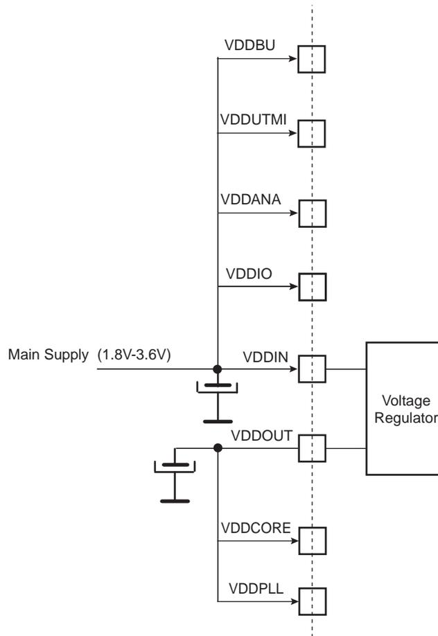
Note: Restrictions: With Main Supply < 3V, some peripherals such as USB and ADC might not be operational. Refer to the DC Characteristics of the product for actual possible ranges for such peripherals.
