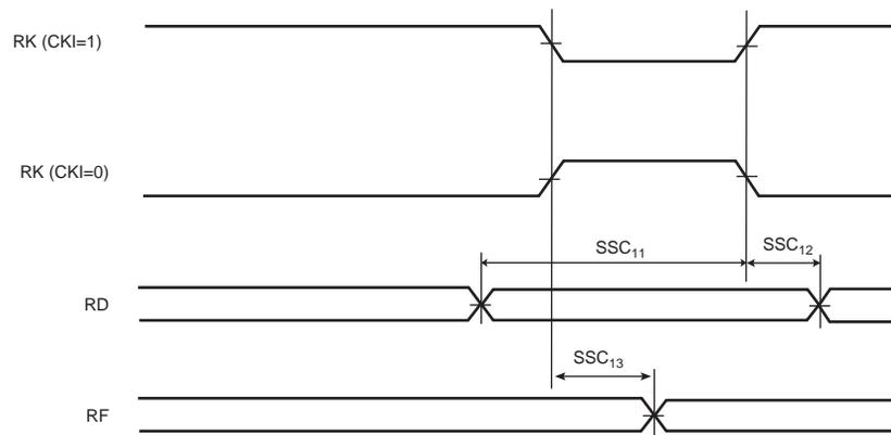
Figure 46-26. SSC Receiver, RK as output and RF as input
