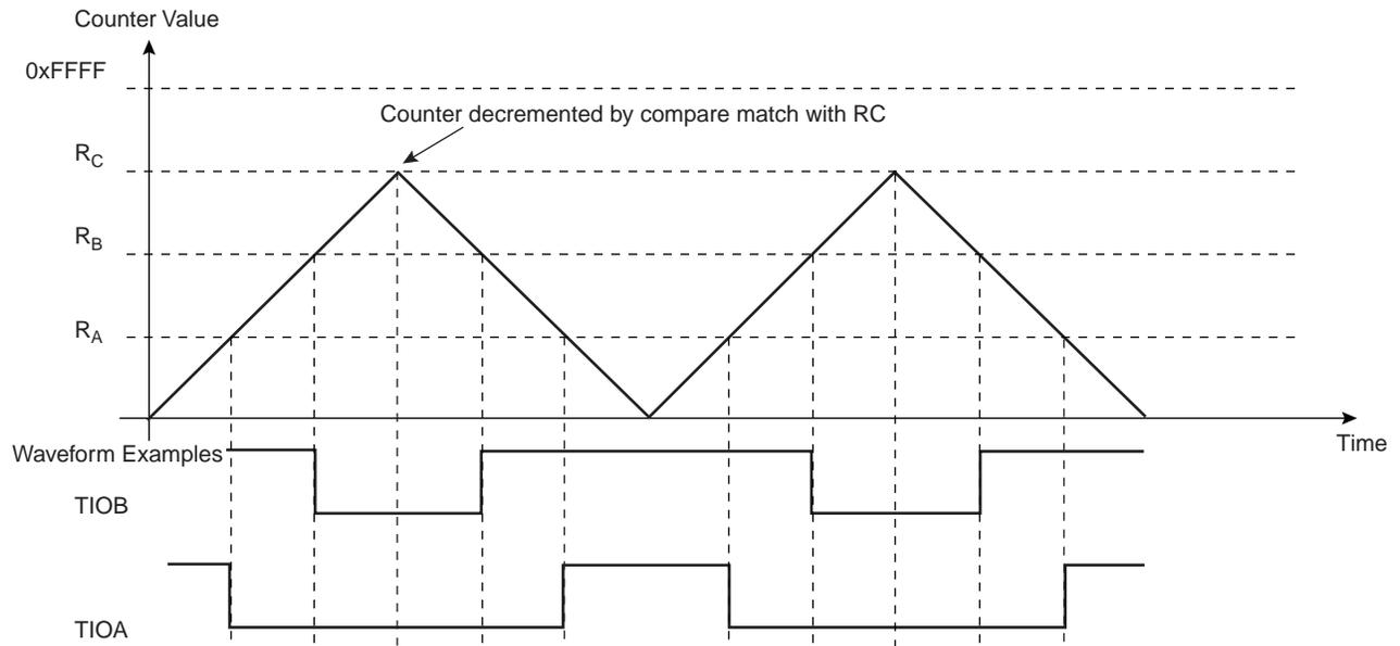
**Figure 37-14. WAVSEL = 11 With Trigger**
