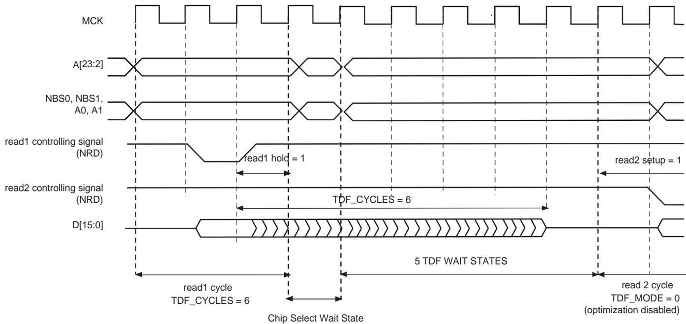
**Figure 27-21.** TDF Mode = 0: TDF wait states between a read and a write access on different chip selects
