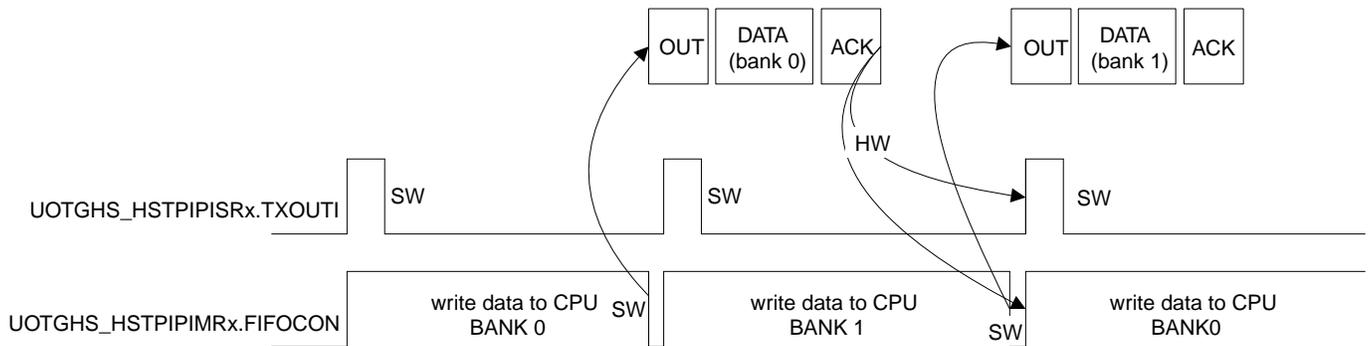
**Figure 40-28.** Example of an OUT Pipe with two Data Banks and a Bank Switching Delay
