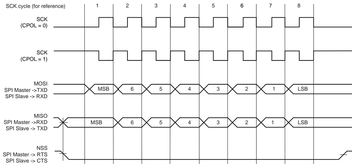
**Figure 36-39. SPI Transfer Format (CPHA=0, 8 bits per transfer)**
