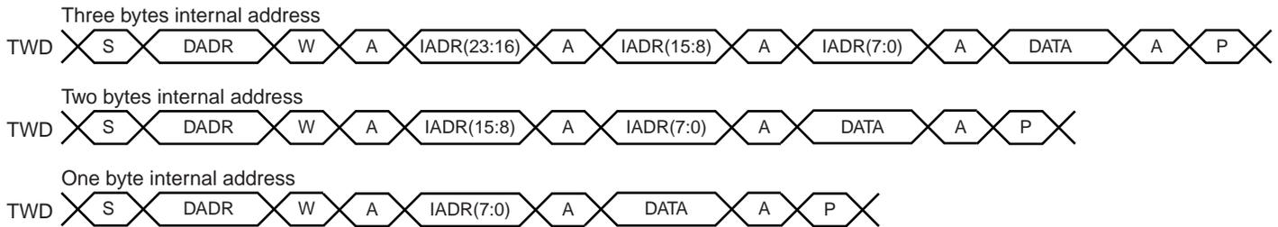
**Figure 34-12. Master Read with One, Two or Three Bytes Internal Address and One Data Byte**
