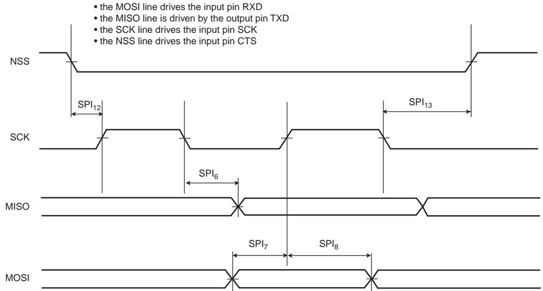
**Figure 46-32. USART SPI Slave mode (Mode 0 or 3)**
