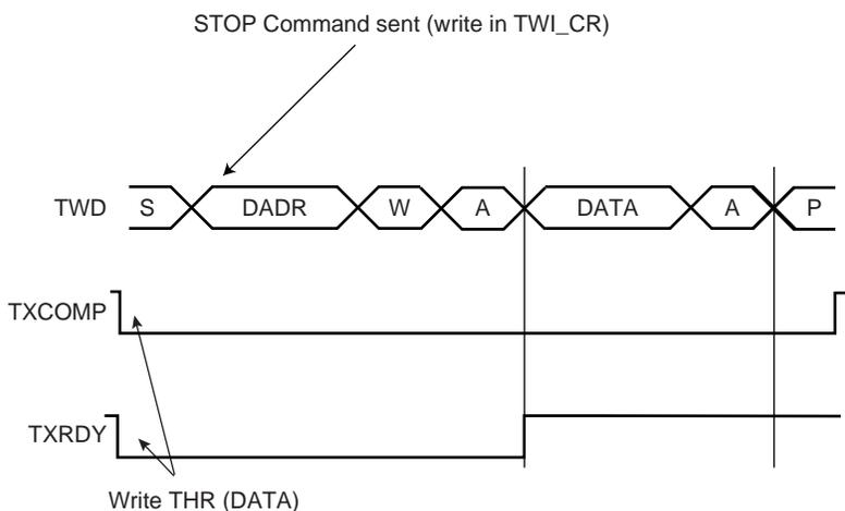
**Figure 34-7.** Master Write with Multiple Data Bytes
