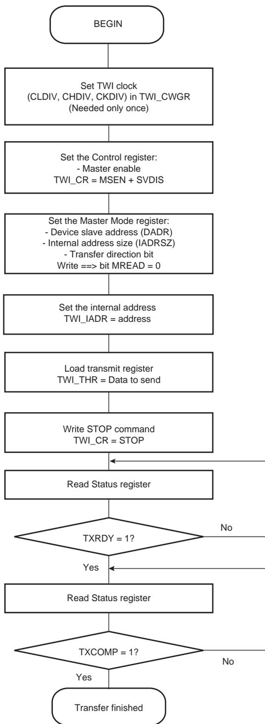
**Figure 34-17.** TWI Write Operation with Multiple Data Bytes with or without Internal Address
