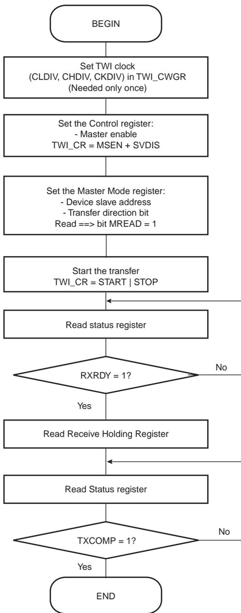
**Figure 34-19.** TWI Read Operation with Single Data Byte and Internal Address
