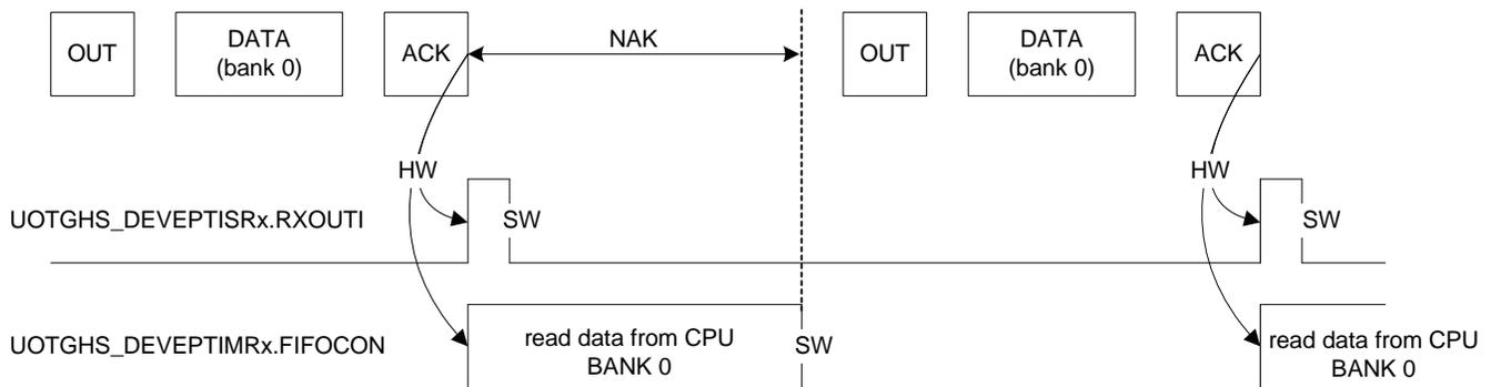
**Figure 40-20.** Example of an OUT Endpoint with two Data Banks
