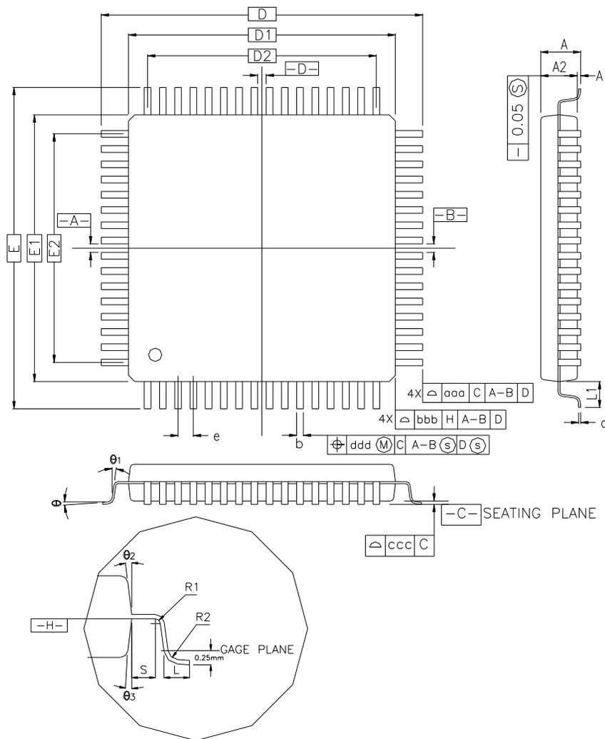
COTROL DIMENSIONS ARE IN MILLIMETERS.
