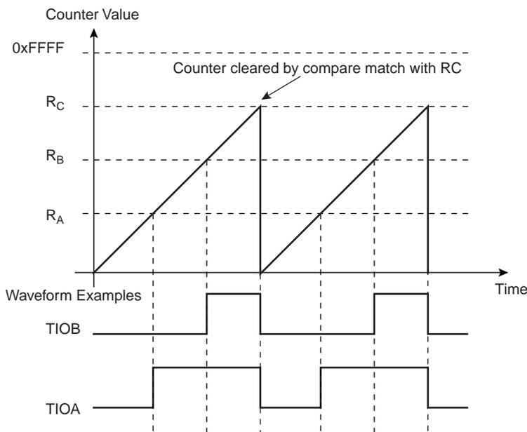
**Figure 37-10. WAVSEL = 10 With Trigger**
