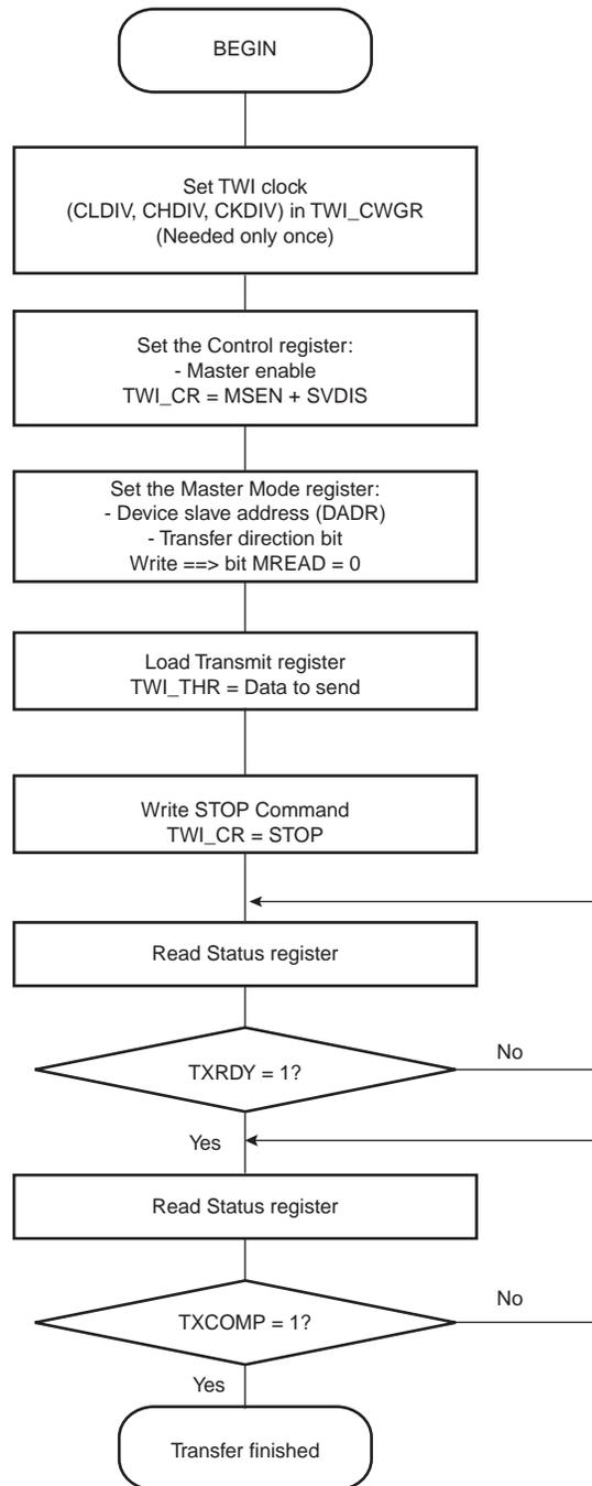
Figure 34-16. TWI Write Operation with Single Data Byte and Internal Address
