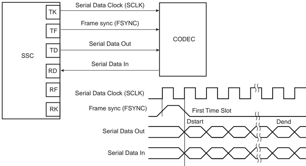
Figure 31-19. Time Slot Application Block Diagram
