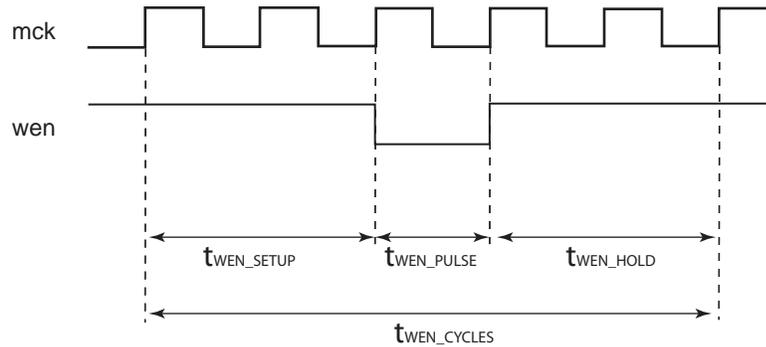
**Figure 27-33.** Write Enable Timing for NAND Flash Device Data Input Mode.
