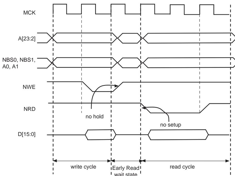
**Figure 27-15.** Early Read Wait State: NCS Controlled Write with No Hold Followed by a Read with No NCS Setup
