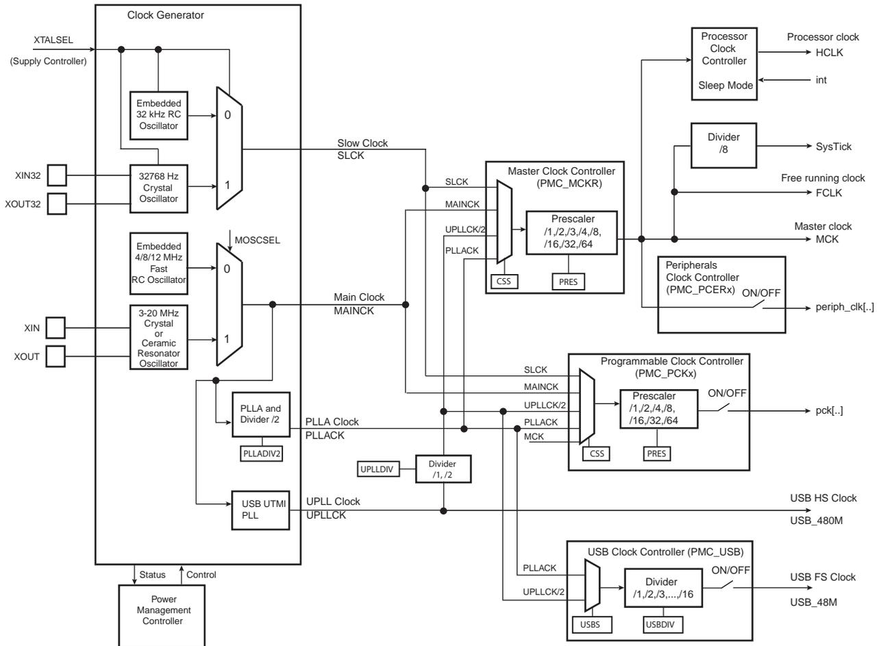
Figure 29-7. Peripheral Clock Divider Block Diagram
