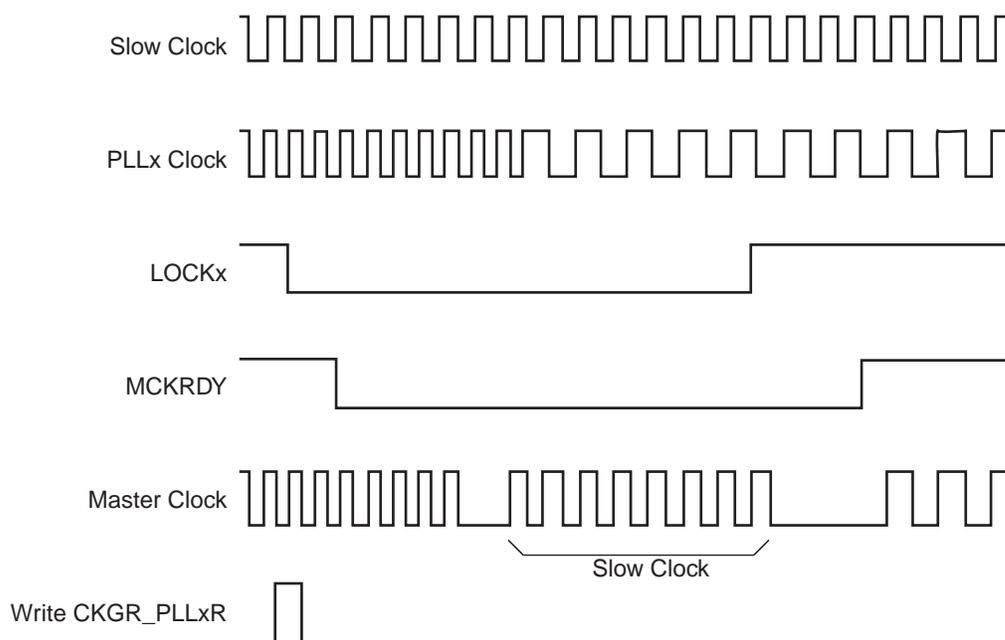
**Figure 29-13.** Programmable Clock Output Programming
