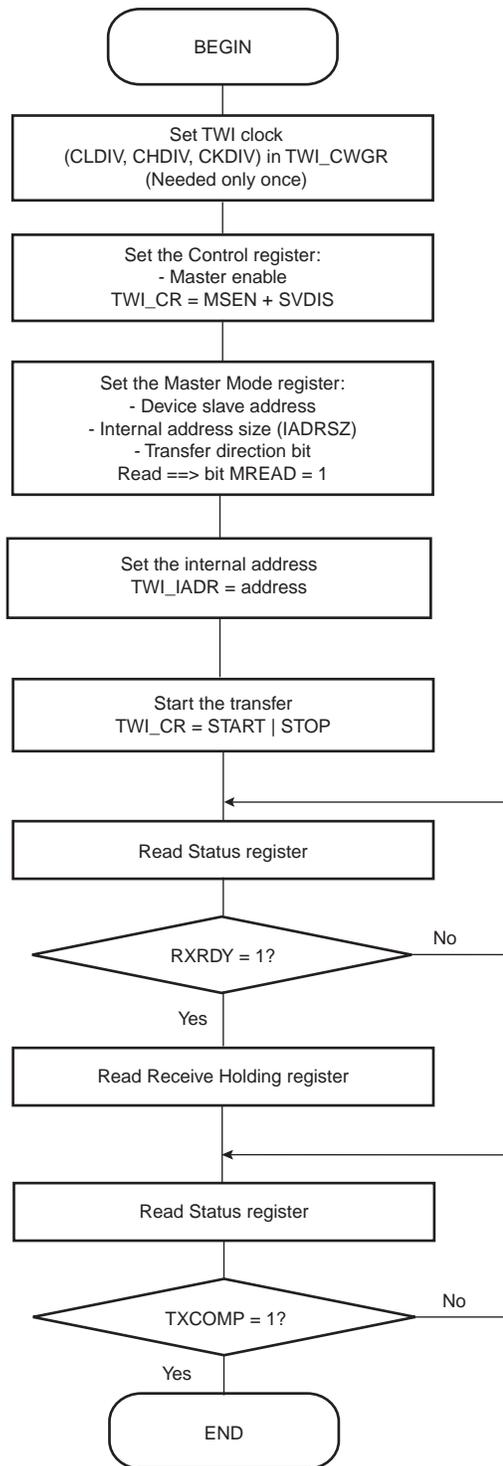
Figure 34-20. TWI Read Operation with Multiple Data Bytes with or without Internal Address
