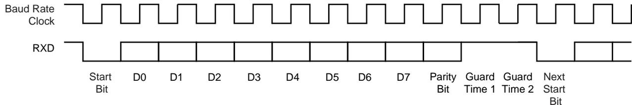
**Figure 36-32.** T = 0 Protocol with Parity Error
