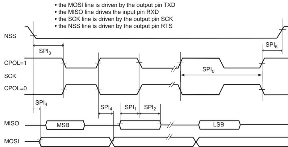
**Figure 46-31. USART SPI Slave mode (Mode 1 or 2)**
