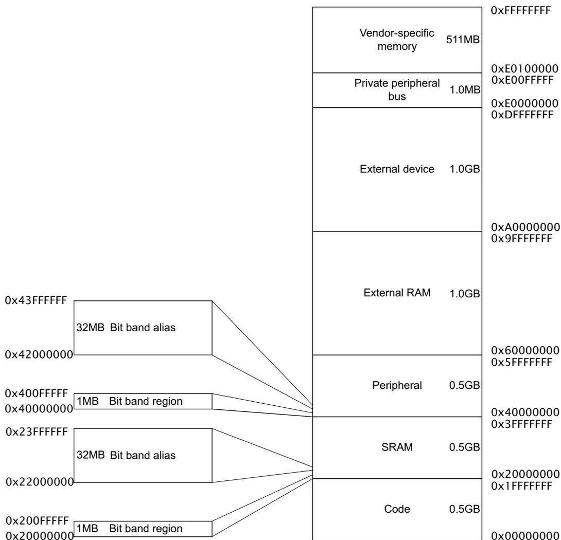
The regions for SRAM and peripherals include bit-banding regions. Bit-banding provides atomic operations to bit data, see “Bit-banding” on page 75.
