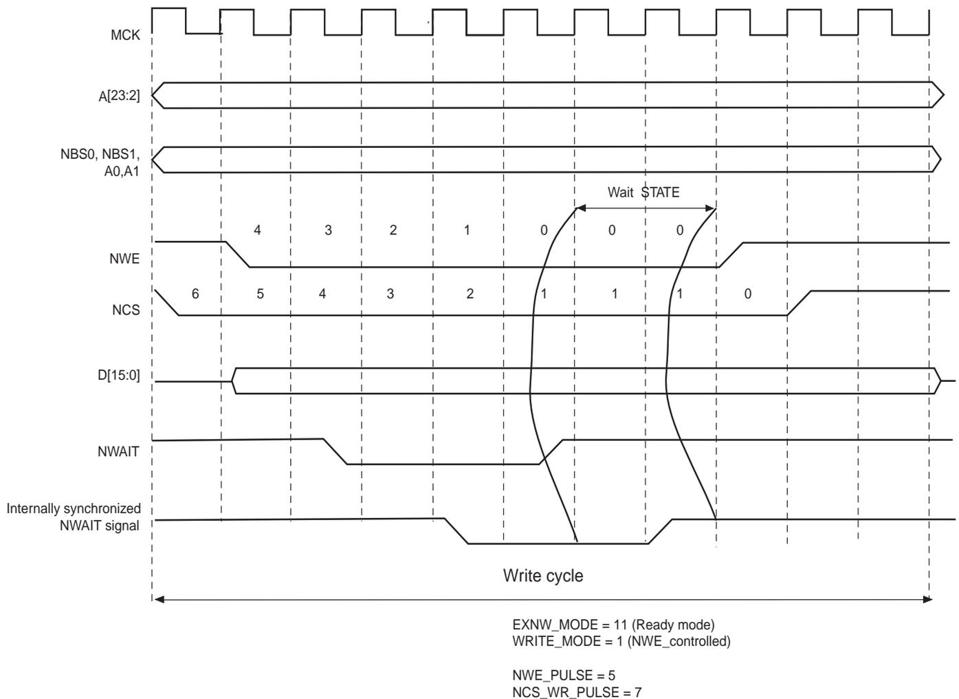
**Figure 27-26. NWAIT Assertion in Read Access: Ready Mode (EXNW\_MODE = 11)**
