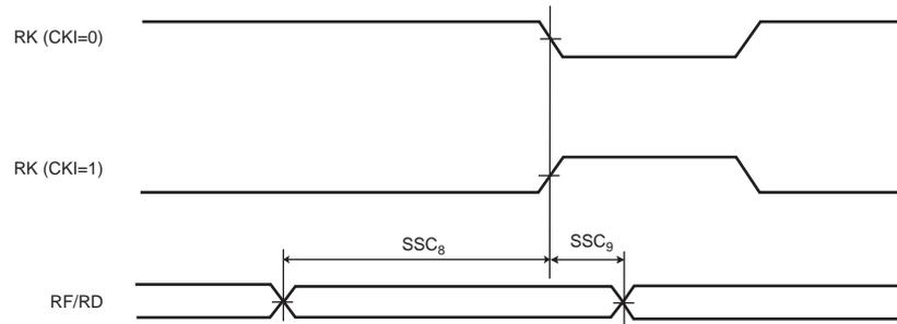
**Figure 46-24.** SSC Receiver, RK as input and RF as output
