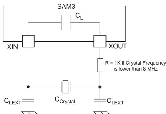
$$C_{LEXT} = 2x(C_{CRYSTAL} - C_L - C_{PCB}).$$
