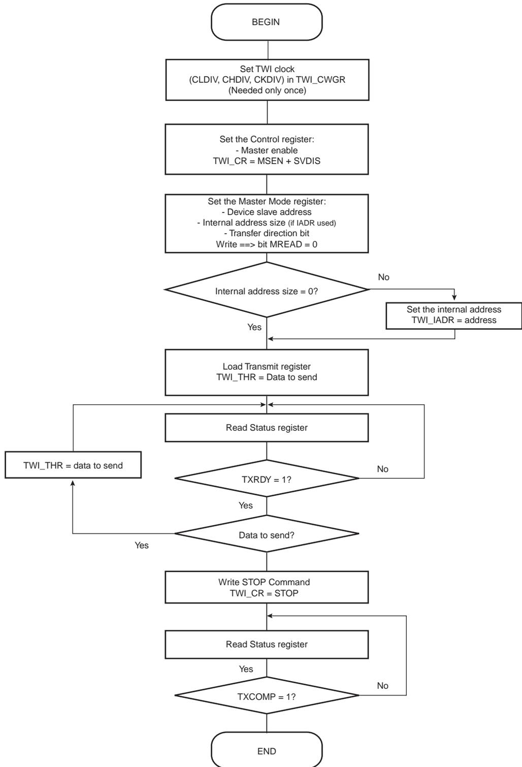
Figure 34-18. TWI Read Operation with Single Data Byte without Internal Address
