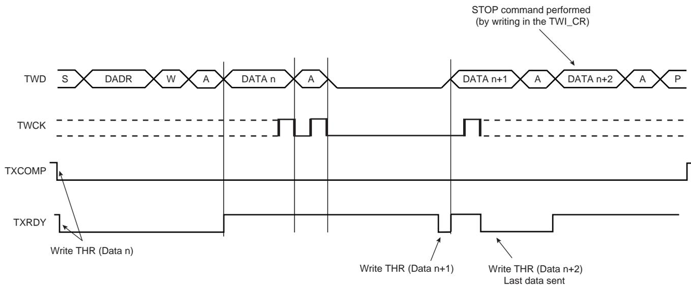
**Figure 34-8.** Master Write with One Byte Internal Address and Multiple Data Bytes
