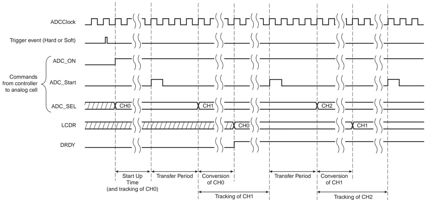
Figure 44-3. Sequence of ADC conversions when Tracking time < Conversion time
