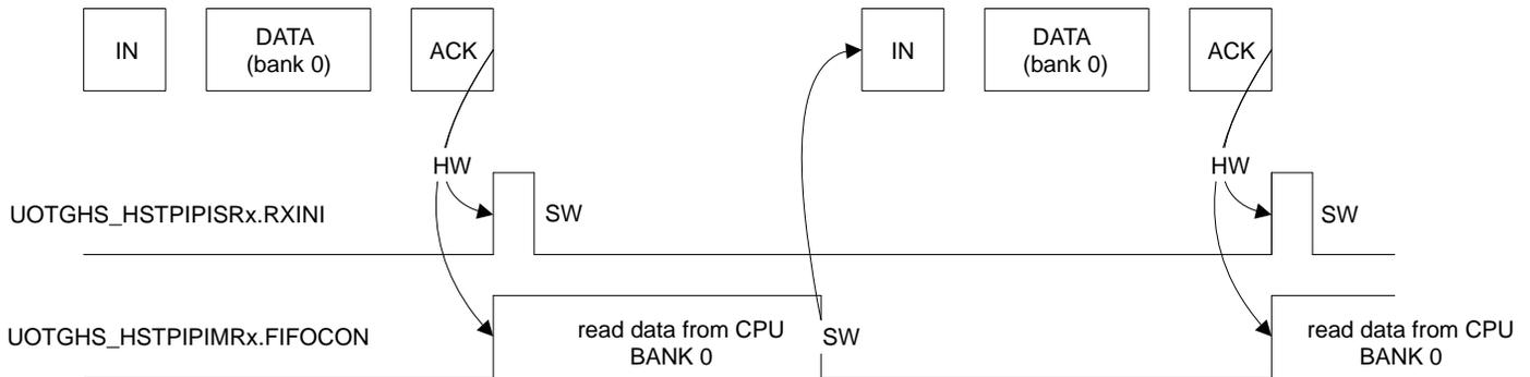
**Figure 40-25.** Example of an IN Pipe with 2 Data Banks
