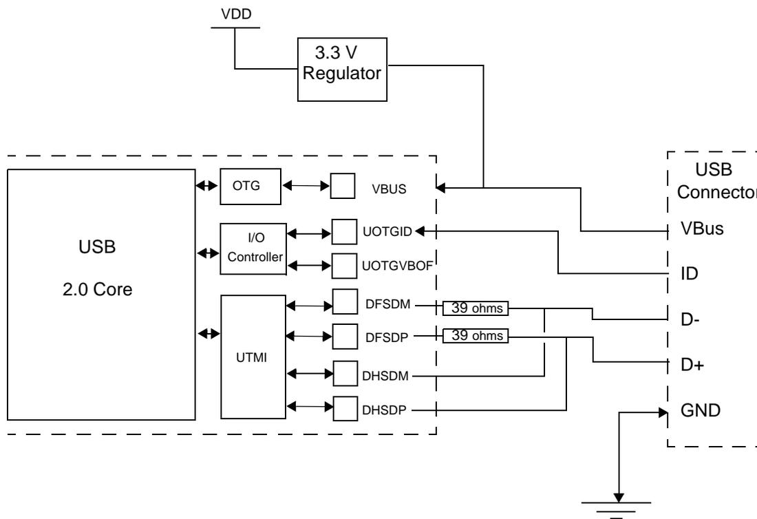
**Figure 40-3.** Self-powered Device Application Block Diagram
