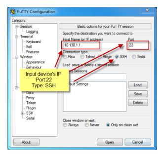
IP address: IP address of LG308
