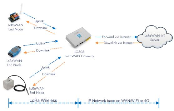
This chapter describes how to use LG308 to work with <u>TTN LoRaWAN Server</u>. The method to work with other LoRaWAN server is similar.
