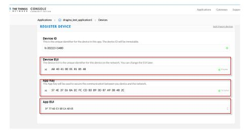
**Step 2**: Power on LT and it will auto join to the TTN network. After join success, it will start to upload message to TTN and user can see in the panel and analyze the data
