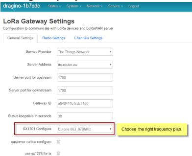
After doing above LG308 will be able to act as LoRaWAN. Below section shows how to add a LoRaWAN End device in this LoRaWAN network and see the data from TTN.
