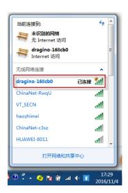
Note: If device has been configured to work in WiFi Client Mode, the WiFi AP mode will be disable and user can't see the dragino wifi SSID.
