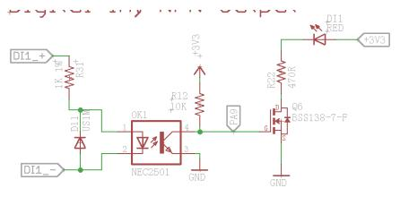
When use need to connect a device to the DI port, both DI1+ and DI1- must be connected.
