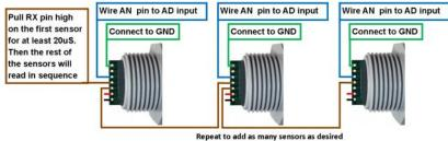
The next method is AN Output Constantly Looping. The first sensor will range, then trigger the next sensor to range and so on for all the sensor in the array. Once the last sensor has ranged, it will trigger the first sensor in the array to range again and will continue this loop indefinitely. Below is a diagram on how to set this up.
