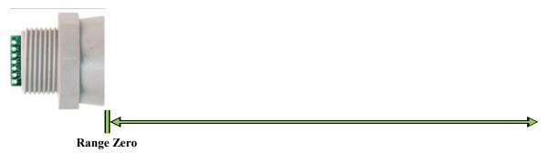
The range is measured from the front of the transducer to the target.
