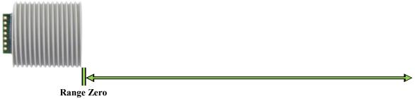
The range is measured from the front of the transducer to the target.
