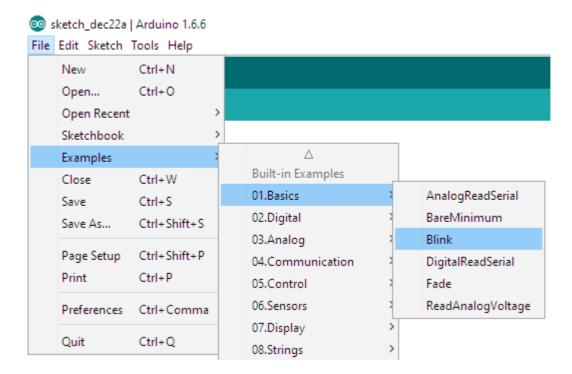
A new window with code would open. Edit the code in order to reflect the hardware of ESP8266-EVB boards. By default, the example assumes the LED is connected to hardware pin #13 (like in most Arduino boards). In our case the LED is connected to hardware pin #5. This information can be acquired from the schematic of the board. Replace all occurrences of "13" with "5". The code should look as follows:
