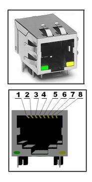
The two leds on the front side of the LAN connector show the state of the Ethernet. The meaning behind the different states can be found in the table below:
