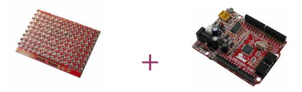
For the LoL Shield to work, It needs to be connected to a board like the olimexino-328. The olimexino-328 is an arduino-like borad, which runs programs called "sketches". The programs themselves are written in C and compiled in the Arduino environment and then uploaded to the board's memory via miniUSB.
