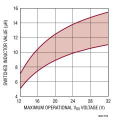
Figure 3. 7.2V at 1.5A Switched Inductor Values
